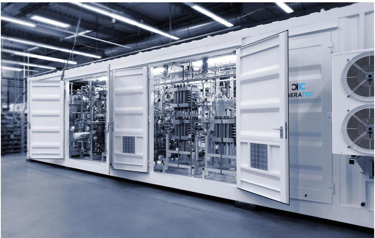
**Figure 2 – An industrial-scale container size Power-to-Liquid plant module (refer to Step 4 in Figure 1) by INERATEC**
