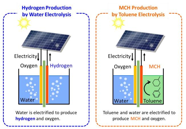
Overview of Direct MCH electrochemical synthesis (Direct MCH®)
