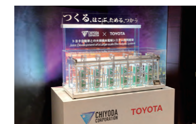
A model of the water electrolysis system. The green area is the 'water electrolysis cell stack' developed by Toyota.
